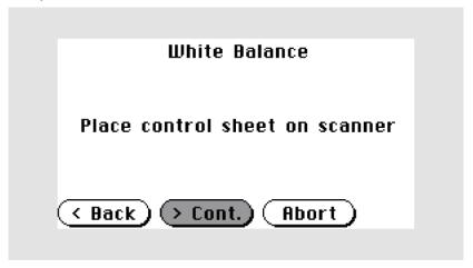
The white balance starts and the calibration is performed. During the white balance, a rotating icon appears. The test target is transported forward and returned. The entire white balance sequence takes about 50 seconds.
