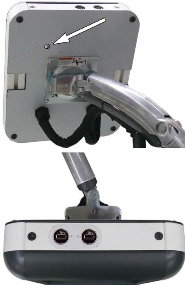
**Picture 4 USB connectors and standby button**
